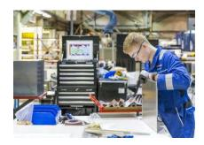
For the most of the time a technician works at his <u>work desk</u>. That's a quite solid table, where he can store his tools in the <u>drawers</u>, fix workpieces by a vice, lay down objects onto the <u>desktop</u>, can lock-up parts inside <u>lockers</u> or collect small parts in <u>utility boxes</u> or store larger parts in <u>shelves</u>.
